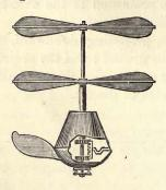
This revolving of the propellers in opposite directions keeps the car from gyration.
